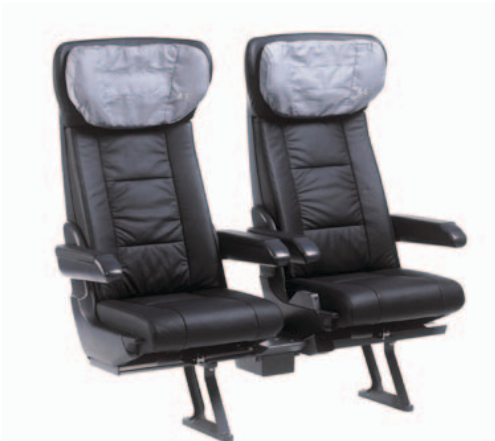
For first-class railcars' tough, new seat back shells and side panels, Grammer Railway Interior GmbH has selected SABIC's new LEXAN FST copolymer – which meets requirements for the highest hazard level (HL3) for R6 under Europe's EN 45445-2 harmonized standard for fire safety.
