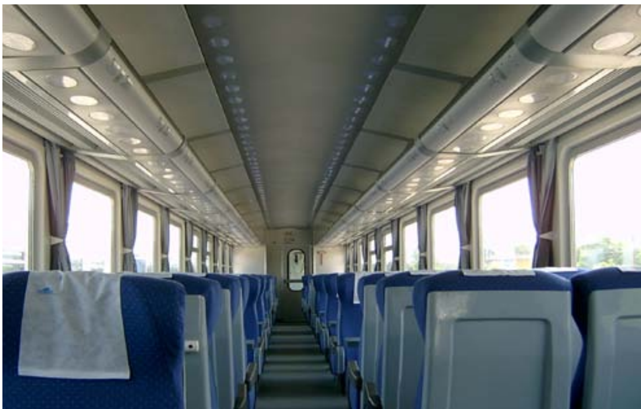
Masterplex selected LEXAN sheets to create the Italian railway's most challenging interior feature, a train ceiling complete with light diffusers.
